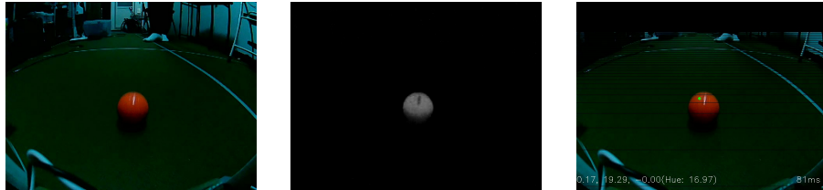
(a) The raw image from the camera. (b) The difference between Cb and Cr signals. (c) The estimated position of the ball.
